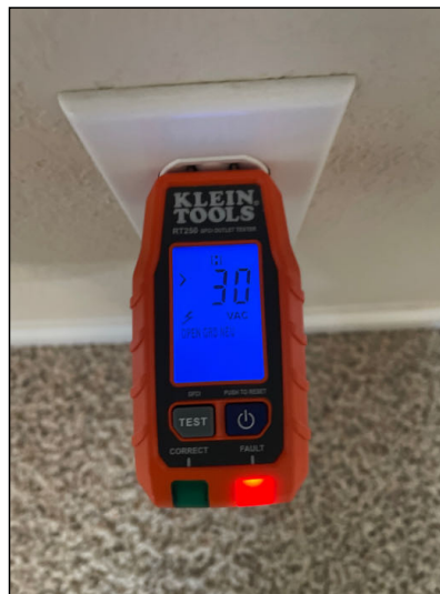
Open Ground showing only on the top portion of the receptacle underneath the window in the living room.
